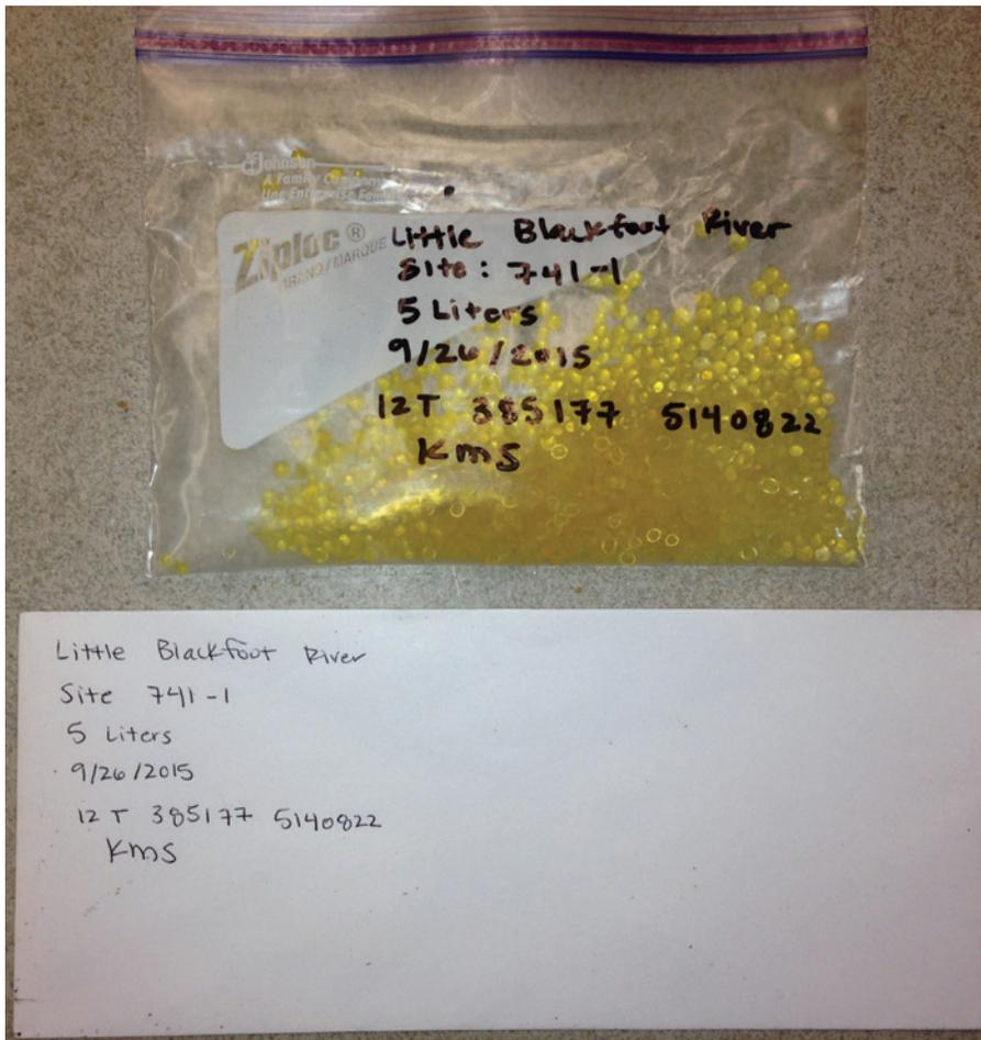
Figure 6—An example of a properly labeled sample.
