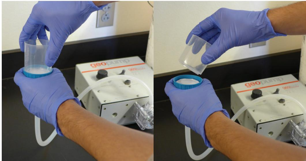
**Figure 4**—Removing the cup from the filter assembly.
